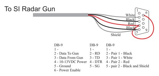
NOTE: The power enable indicates that the cable is plugged in to the charger and that the charger and RF transmitter should be powered.
